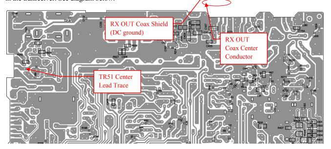
17) Locate the Yellow wire from the RFX85 and route it through the slot on the transceiver's PCB where TR43 and TR56 were removed. On the solder side of the transceiver PCB, solder the Yellow wire to the trace at the positive side of C164. See diagram below.
